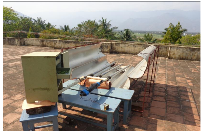
Fig3. Evacuated Tube solar air heater
